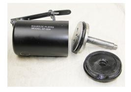
Clean the inside of the power pack housing to remove any residual debris and lubricate it with a small amount of light machine oil.
