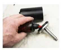
Replace the internal and external O-ring on the housing end cap
