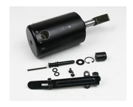
Remove the lever handle from the housing by removing the 2 Phillips screws Tip the housing on its side and tap out the plastic valve spacer, exposing a small snap ring underneath.
