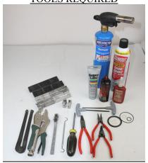
Bench Vise Rubber and aluminum vise pads Wire brushes Vise Grip Spanner wrench Small picks 9/64" Allen Wrench 1/8" Allen Wrench Clamp Blocks for securing shaft assembly in vise Internal & External Snap Ring Pliers (small tips) #2 Phillips Screwdriver Propane Torch Parts Cleaner Loctite 290 (or equal) Light machine oil Light Grease
