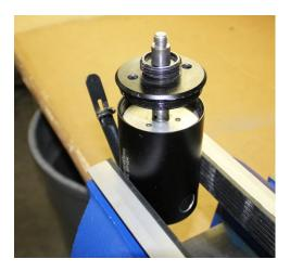
Slowly, remove the shaft and piston plate assembly from the housing. If this assembly is difficult to remove, set your air pressure regulator down to 30-40 psi, and reconnect the air source to the tool and activate the lever valve. The compressed air will assist in removing the piston assembly. Once removed, disconnect your air source from the tool.
