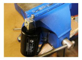
Remove the tool and shaft clamp block from the vise.
